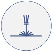
This method is achieved by burning the top layer of the substrate with a thin laser beam that cuts through the product creating a lasting detailed logo.
