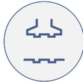
Deboss printing involves creating a die in the shape of a logo that is pressed into the surface creating a permanent sunken design.
